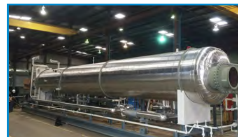
60 GPM Gas Sweetening and Hydrocarbon Dew Point Package, Pakistan
